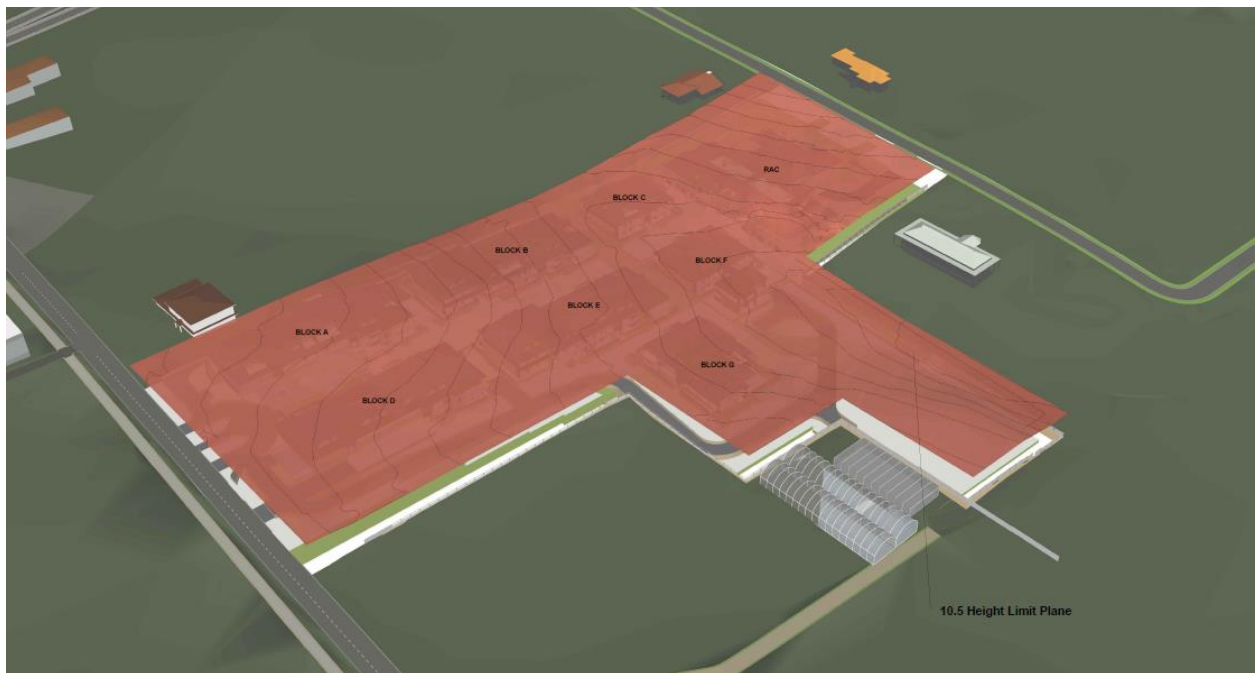
Figure 5 Height Plane diagrams of the 10.5m height limit under HLEP 2013 (Source: Marchese Partners)
